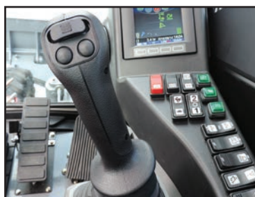
Pilot Operated Controls
