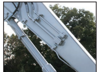
Auxiliary Hydraulic Lines
